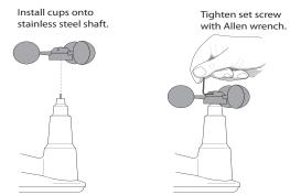
Note: If the wind cups don't spin freely, loosen the set screw, remove the wind cups from the shaft, and repeat the installation steps.
