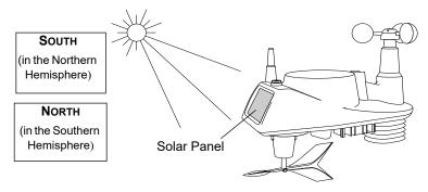
Note: The wind direction is calibrated assuming the solar panel is facing south. If you install the sensor suite with the solar panel pointing in a direction other than south, you will need to use the wind direction calibration function in the WeatherLink Console in order to obtain accurate wind direction readings. See *WeatherLink Console User Guide* for more information.
