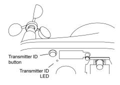
Unless you have intentionally changed your transmitter ID, the LED should blink *one time* because the default transmitter ID for the sensor suite is 1. If you have changed the ID, the LED should blink the number of times equal to the ID you have set (i.e., twice for an ID of 2, three times for an ID of 3, etc.).
