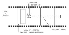
If placing the #1986 in the center channel you may need to cut an opening from the outside to be able to tighten down the nuts and secure the wire or use longer bolts and spacers.
